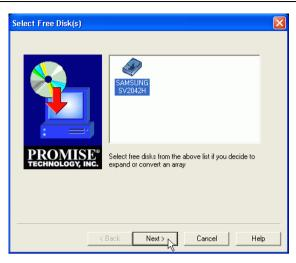
Figure 63. Select a disk drive to add to the array.
